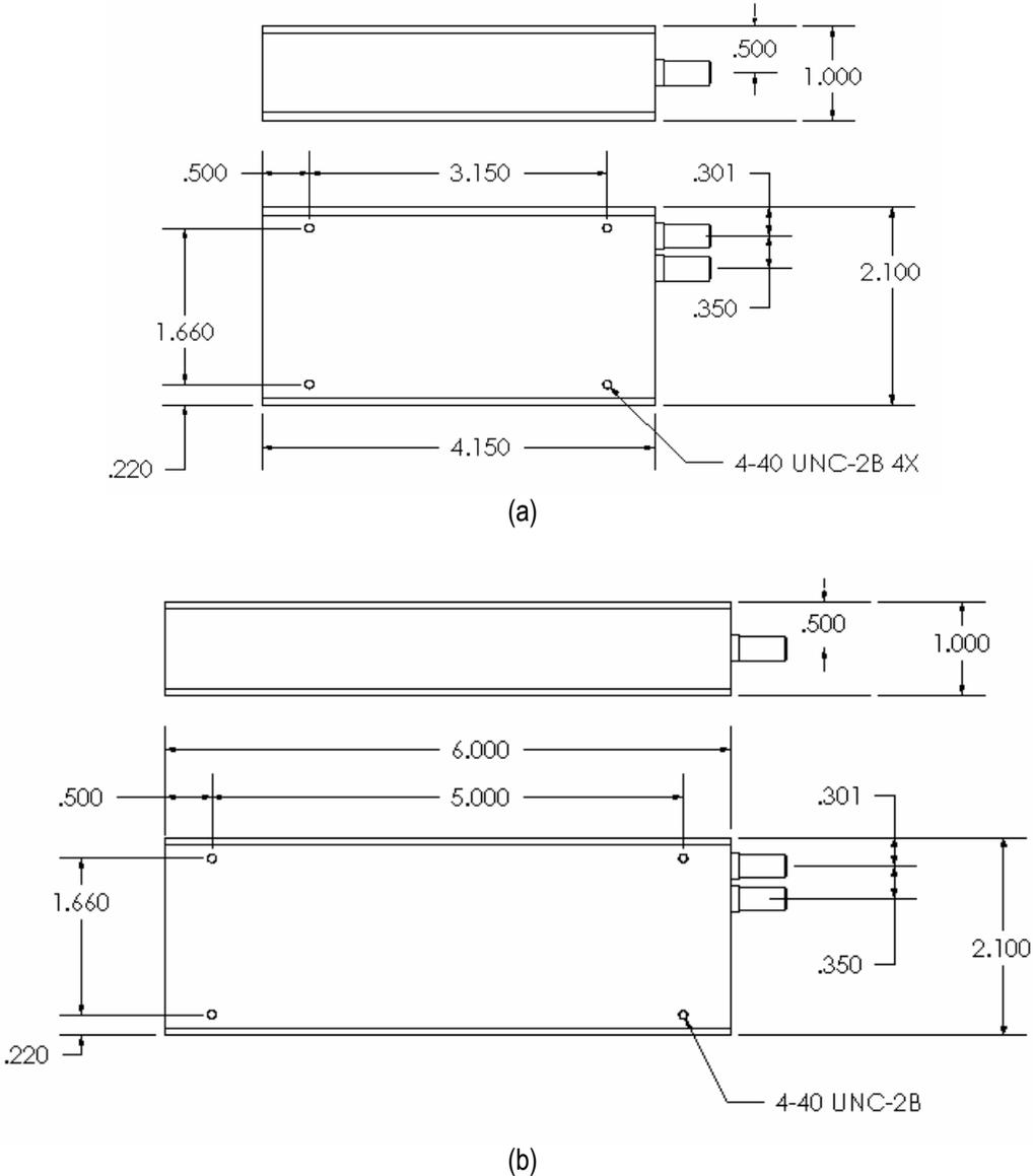
Figure 2. Mechanical layout of the F-VDL manually variable optical delay line: (a) 330 ps model, and (b) 600 ps model
