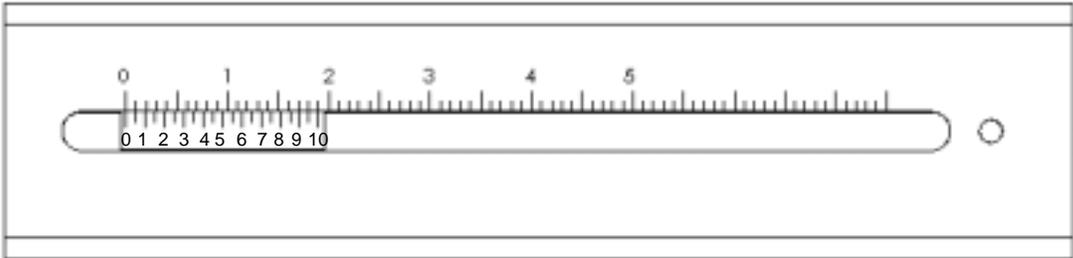
Figure 3. Delay length change ruler for the F-VDL device. The marked unit in the stationary scale is in centimeters with millimeter subdivisions.
